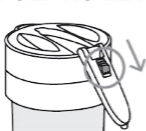
Pull downward to unlock handle
