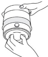
Other hand hold and pull on top of the kettle
