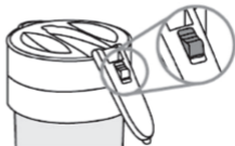
Push upward to lock the handle
