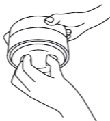
Grab and pull down from base holding position
